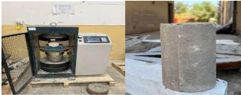
Figure 4.4: Tensile testing setup for cylindrical concrete samples.
